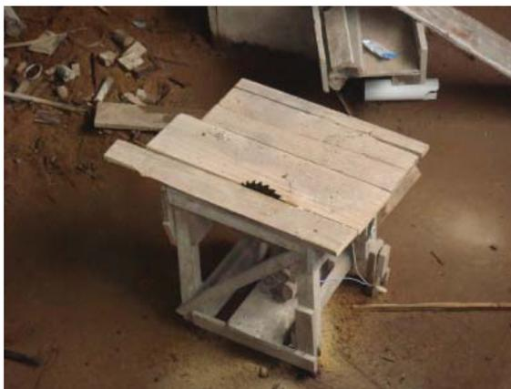
Figura 22 – Serra circular montada
